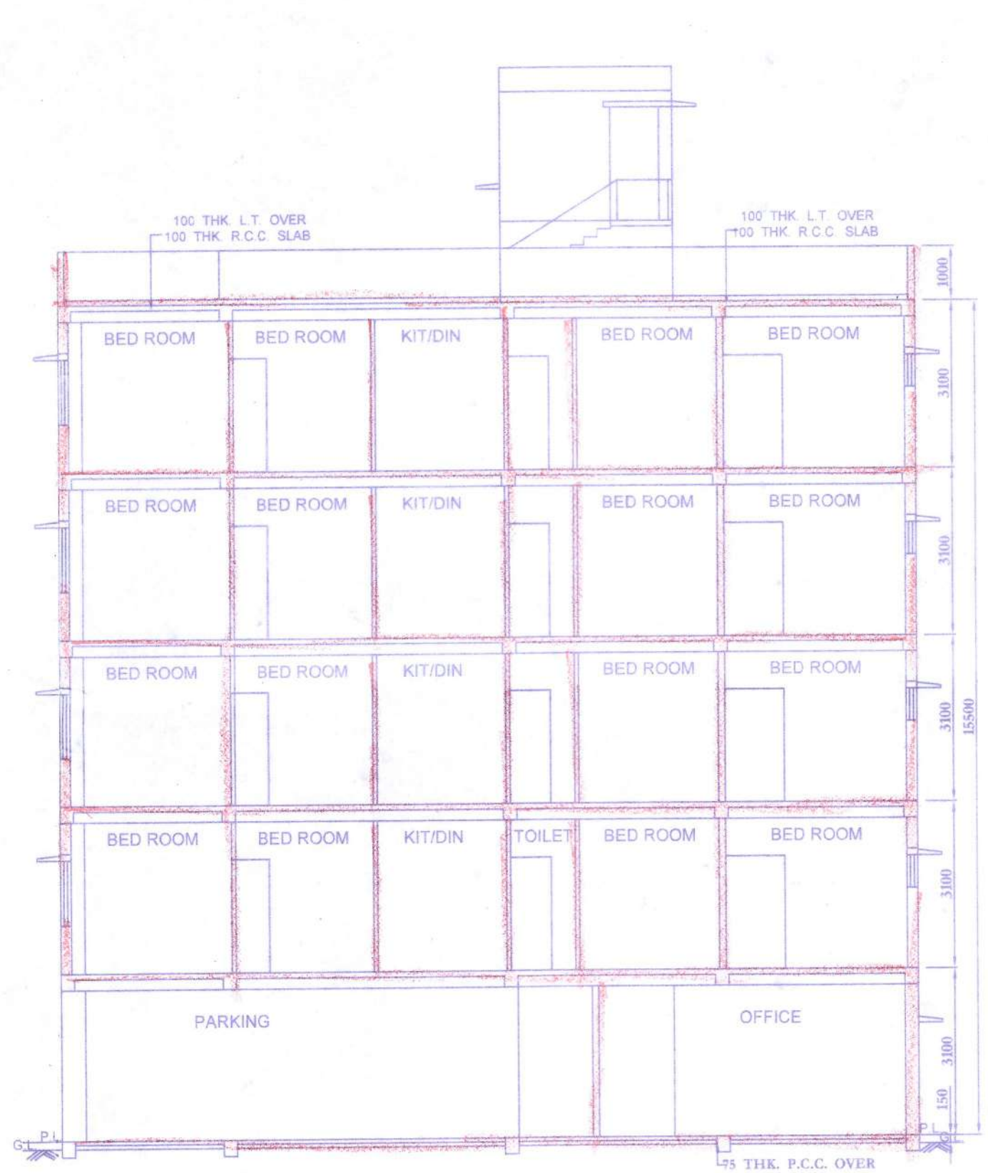
SECTION AT A-B SCALE - 1:100
